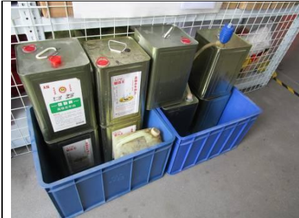
Image 25: Secondary containers were provided to all chemicals to prevent from leakage.
