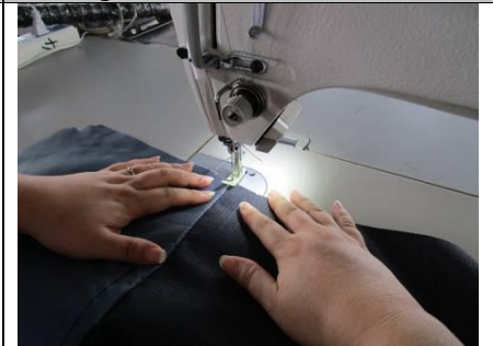
Image 21: Needle guards were installed on all sewing machines.
